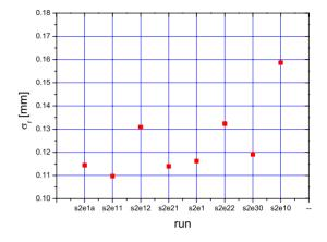
Figure 8: The transverse radiation size at the location z = -6 m for examined cases.
