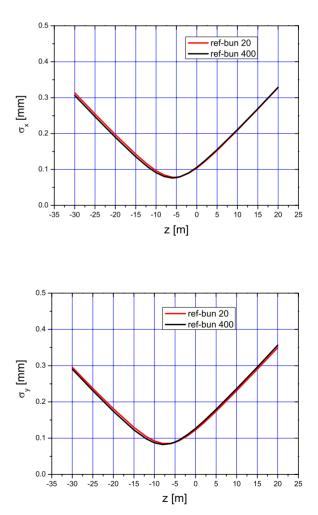
Figure 3: A comparison between calculations with 20 and 400 slices using the Fourier optic method. Using the electric field distribution of 20 slices describes the radiation field almost as good as using 400 slices.
