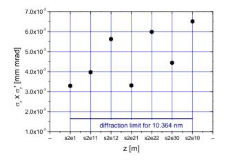
Figure 7: The phase space volume using the GENESIS output for the examined cases at the end of the final amplifier is shown. The phase space volumes are too large as expected.
