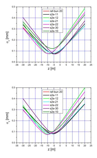
Figure 5: The horizontal and vertical waists of the examined cases are shown compared to the reference bunch. The deviation from the nominal beam size amounts to 56% horizontally and 13% vertically.
