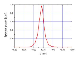
Figure 1: The average spectral power for the start-to-end simulations including error sources from injector and linac is shown.
