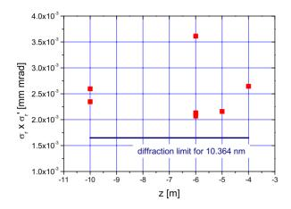
Figure 6: The phase space volume as a function of the waist location for the examined cases. The theoretical value for adiffraction limited photon beam is shown for comparison.
