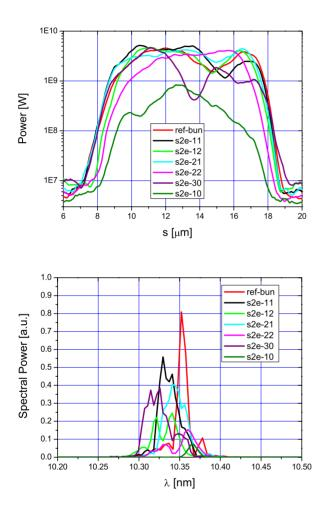
Figure 2: Power and spectral distribution of the reference bunch, and the examined cases, named by their start-to-end bunch number are shown.
