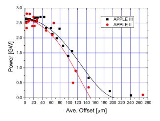
Figure 4: The output power of the final amplifier as a function of average module-offset after 15 m for APPLE-II and APPLE-III devices. The lines are included to guide the eye.
