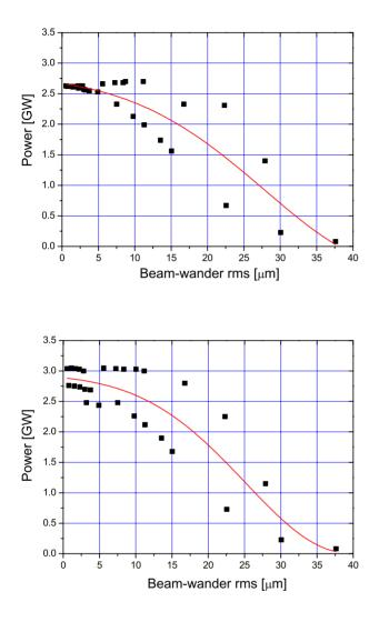
Figure 7: The output power as a function of the beam wander, without (top) and with (bottom) an additional field error of  $2 \times 10^{-3}$  for the APPLE-III device. From the results of the many sets of the randomly distributed module offsets, only upper and lower limit are shown. The lines are included to guide the eye.
