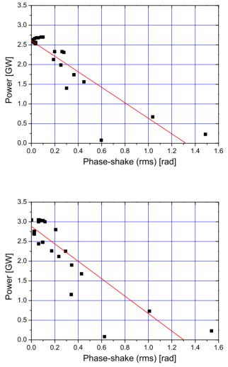
Figure 6: The output power as a function of the phase shake, without (top) and with (bottom) an additional field error of  $2 \times 10^{-3}$  for the APPLE-III device. The lines are included to guide the eye.
