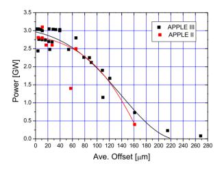
Figure 5: The output power of the final amplifier as a function of average module-offset after 15 m. A relative correlated field error of  $2 \times 10^{-3}$  was included in addition. The lines are included to guide the eye.
