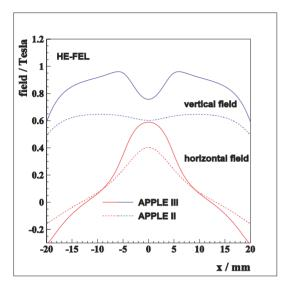
Figure 2: Transverse field profiles for the HE-FEL evaluated for an APPLE-II design (dashed line) and APPLE-III (solid line). The vertical field (blue) is calculated at row shift of 0 and the horizontal field (red) at row shift =  $\lambda_u/2$ .
