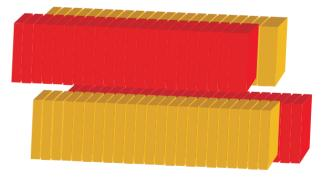
Figure 1: The APPLE undulator consists of four rows of magnets. Variable polarization can be provided by shifting the rows. Shown is an antiparallel shift resulting in tilted linearly polarized radiation.
