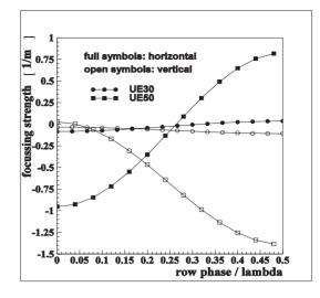
Figure 3: Focussing of the final amplifier of the HE-FEL at the smallest gap in the parallel mode.
