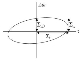
Figure 1: Region of phase space occupied by radiation,  $\Delta a = a - a_r$ .
