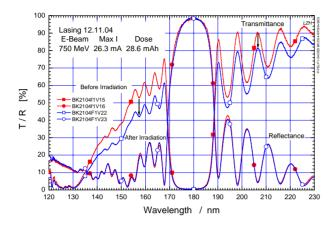
Figure 2. Spectral behaviour (reflectivity and transmittance) of the front optical cavity mirror before and after the first lasing experiment (received dose corresponding to an integrated current of 29 mAh).
