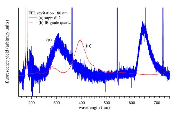
Figure 3. Fluorescence signal from suprasil 2 (a) and infrared grade quartz (b) specimens using the FEL at 180 nm as excitation source.
