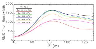
Figure 8: *GINGER* predictions for RMS inverse spectral bandwidth vs. *z* for a 200-pC bunch charge propagating in a Cu vacuum chamber for various compensation tapers.
