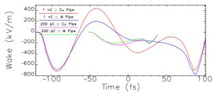
Figure 3: Total longitudinal wake for Cu & Al vacuum chambers for 1-nC and 200-pC bunch charges.
