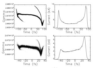
Figure 1:  $t - \gamma$  scatterplot and I(t) at undulator entrance for the 1-nC and 200-pC microbunch charge cases.
