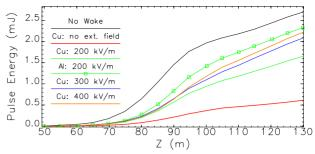
Figure 5: Pulse energy vs. z as predicted by *GINGER* for a 1-nC bunch charge in Al & Cu vacuum chambers for several wake compensation undulator strength tapers.
