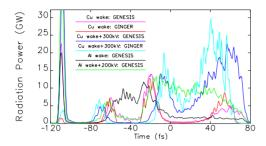
Figure 4: Predicted instantaneous power (artifically smoothed to 1-fs resolution) at  $z=100\,\mathrm{m}$  for a 1-nC bunch charge propagating in a Cu vacuum chamber with and without wake effects.
