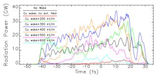
Figure 6: GINGER predictions for instantaneous power at  $z=130\,\mathrm{m}$  for a 200-pC bunch charge propagating in a Cu vacuum chamber for various degrees of wake compensation tapers.
