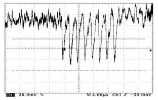
Figure 1: Signal from a Pyroelectric sensor for 8 subsequent bunches of 1nC charge in first spectroscopic order. The wavelength range covered by the detector is about  $40 \mu m$ .
