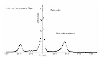
Figure 3: TG-Spectrometer is illuminated by CDR and a  $357 \mu m$  band-pass filter is in the front of the detector.
