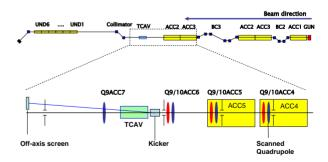
Figure 1: Sketch of the VUV-FEL beam line and the part used for the experiment. The beam passes a transverse deflecting cavity (TCAV) streaking it vertically and gets horizontally deflected by a kicker onto an off-axis OTR monitor. The Quadrupole Q9ACC4 is used for scanning.
