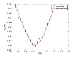
Figure 3: Measured and reconstructed horizontal bunch sizes for different quadrupole currents.
