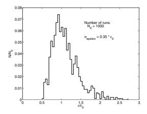
Figure 8: Result of a Monte Carlo simulation for the reconstruction of the emittance with random quadrupole strengths as specified in the text. The emittance values  $\epsilon$  are normalized to the value  $\epsilon_0$  obtained for the default quadrupole strengths.
