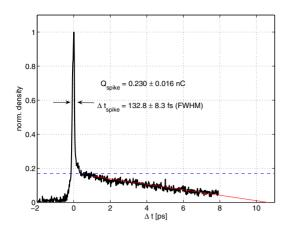
Figure 5: Measured longitudinal density profile. The charge density is normalized to its peak value. The region with densities larger than the threshold given by the dashed blue line defines the spike. The red line is a simple approximation for the part of the bunch that didn't hit the monitor.
