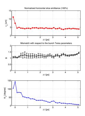
Figure 6: Horizontal slice emittance  $\epsilon_x$ , mismatch parameter B and mismatch phase  $\Theta_x$  along the bunch.  $\Delta t=0$  refers to the peak density in the vertical profile. Mismatch parameter and phase are calculated with respect to the Twiss parameters of the total bunch. The error bars refer to statistical errors only.
