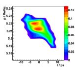
(c) measured longitudinal phase space 3.45 m down-stream from the the cathode
