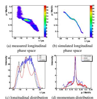
Figure 2: Measured (a) and simulated (b) longitudinal phase space and their projections: longitudinal (c) and momentum (d) distribution for 1 nC bunch charge, optimum launch phase and a flat-top laser distribution with about 20 ps FWHM pulse length. In (c) and (d) the black curves are direct measurements, the red ones are the projections of the measured longitudinal phase space and the blue ones are simulations.
