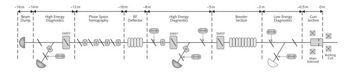
Figure 5: Preliminary layout scheme of the PITZ2 setup.
