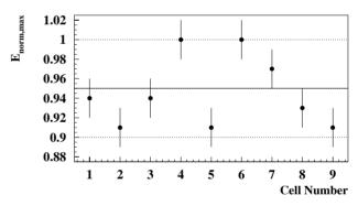
Figure 3: Field flatness obtained as a result of the booster tuning including measurement errors. The maximum field is normalized to 1. The average field is shown as full line.
