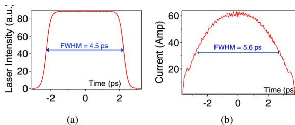
Figure 3: a) Temporal laser profile; b) Longitudinal bunch profile at the exit of SOB.
