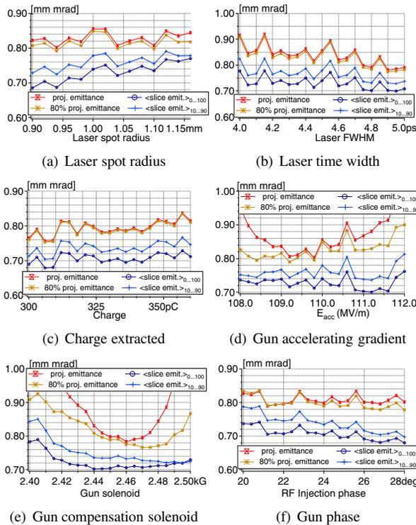
Figure 5: Sensitivity studies: emittance behavior vs. laser and gun parameters.
