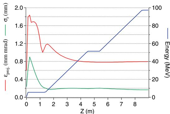
Figure 2: Projected radial emittance, radial spot dimension and energy along the photoinjector beamline
