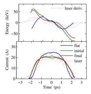
Figure 2: Energy-time correlation and current distribution obtained from the energy spectra shown in Fig. 1. The laser distributions are scaled by 0.5 in time. The dotted lines in the top figure are smoothed derivatives of the laser shapes scaled to match the respective energy correlations.
