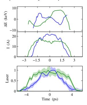
Figure 4: Time distributions from phase space reconstruction of the 70 pC beam. Blue indicates the Gaussian, green the flat-top case. The top panel shows the correlation between slice energy vs. time, the middle shows the current distribution, and the bottom the corresponding UV laser pulse distributions.
