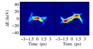
Figure 3: Longitudinal phase space reconstructions for 70 pC. Panel a) shows the Gaussian, b) the flat-top case.
