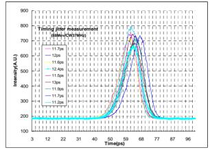
Fig.5. Bunch timing jitter observation for e-beam energy at 88MeV and CW repetition rate 37.4MHz.
