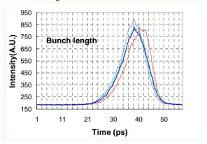
Fig.4. Bunch length measurements from OTS1 for 88MeV beam energy, 9.68MHz CW repetition rate.
