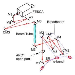
Fig.3. Schematic of the second optical transport system(OTS2). M, flat mirrors. CM, concave mirrors. Detailed description are given in the text.
