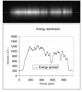
Fig.11. A streak image and the beam energy distribution analysis. The beam configuration is same as (b) in Fig.8.
