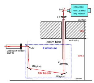
Fig.2. Schematic of the first Optical Transport System (OTS1) after the first dipole. M, flat mirrors. L, lenses.
