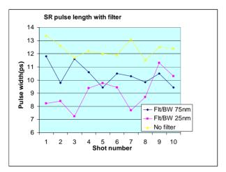
Fig.7. Comparison of bunch length data with and without band-pass filters. E-beam energy is 88MeV, CW beam at 37.4MHz.
