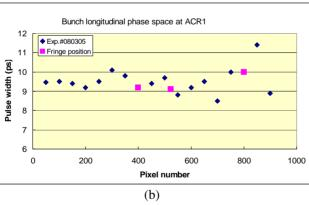
Fig.10. (a) An typical image from streak camera. The numbers along the energy axis are the fringe positions. (b)Analyzed pulse width (FWHM) along the different energy positions. Pixel number corresponds to beam energy spread. The center pixel (512) is approximately the nominal setup beam energy(110MeV).
