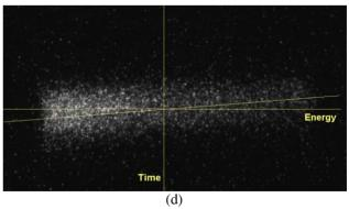
Fig.8. Streak images for different beam setups. Higher energy is at the right of the horizontal axis and the down side of the vertical axis is earlier in time.
