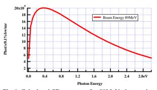
Fig.6. Calculated SR spectrum for 89MeV electron beam in the magnetic dipole. 800nm corresponds to 1.55eV.
