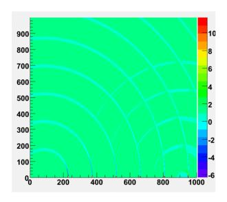
Figure 5. Contour map of  $B_z$  following the predictions of classical electrodynamics. The area shown corresponds to 12 cm in x, and 10 cm in the y direction.
