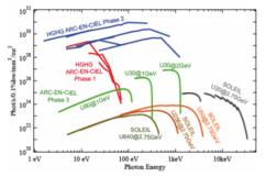
Figure 1 : Peak brilliance. Phase 1 : HGHG radiation + seeding wavelength,  $P_{seed} = 100 \text{ kW}$  for HHG harmonics n°7-9, 600 kW for n°3-5. 1 kA, F= 0.1. Phase 2 :HGHG radiation 1.5 kA, 1.35  $\pi$  mm.mrad, 0.0004% slice energy spread, 200 fs, beta=2 m, F = 0.088. Phase 3 : spontaneous emission of undulators of period 30 and 80 mm calculated with SRW. Undulator period length in mm in ID name.
