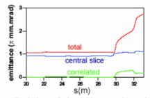
Figure 2 : Evolution of the emittance along the chicane. Chicane parameters: total length: 10 m, R56=0.15 m, dipole length : 0.3 m. First dipole at s=23 m.
