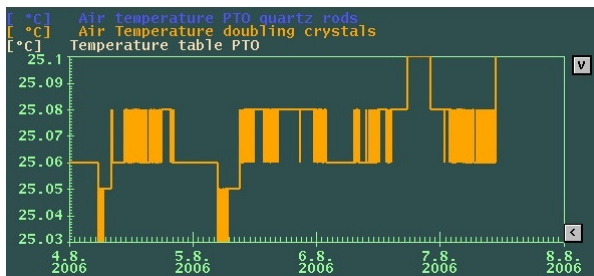
Figure 2: As an example, the air temperature measured at the laser over a period of 3 days. The temperature reading is within \pm 0.02^\circ\text{C} .
