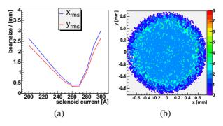
Figure 2: Simulations of the electron beam size as a function of the solenoid current (a) and transverse beam properties at the screen station (b) for a gun and booster phase with maximum energy gain and a flat-top longitudinal laser distribution at 1 nC.
