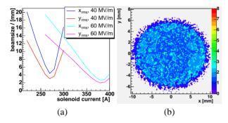
Figure 3: Simulated transverse electron beam size as a function of the solenoid current for 40MV/m and 60MV/m gradient (a) and transverse beam properties at the screen station (b) for a gradient of 40MV/m in the gun and a phase with maximum energy gain, a flat-top longitudinal laser distribution at 1 nC, when the booster is turned off.
