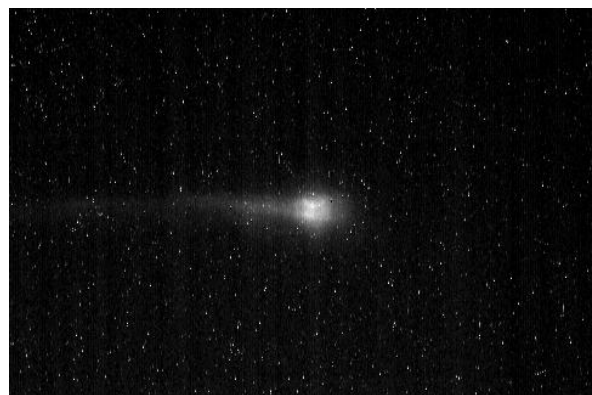
Figure 4: The OTR image of the beam profile measured using a CCD camera. The horizontal direction is the bending orbital plane of the electron beam. Left side of the image is lower momentum one.
