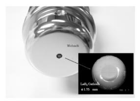
Figure 3: The assembly of single-crystal LaB<sub>6</sub> cathode.
