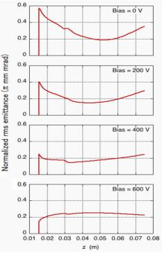
Figure 9: The bias voltage dependence of normalized emittance.
