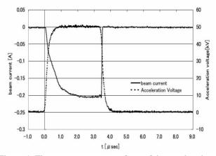
Figure 4: The measurement waveform of the accelerating voltage and beam current.
