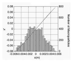
Figure 8: The macro-particle distribution and phase space distribution at the end point according to a simulation with 3D FDTD.
