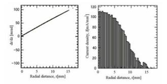
Figure 6: The macro-particle distribution and phase space distribution at the position 200 mm from cathode according to a simulation with KUAD2.
