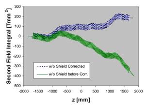
Figure 5: Second field integrals of raw data and corrected data.
