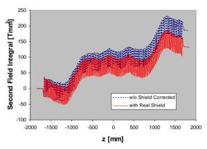
Figure 6: Second field integrals predicted from data without shield (blue broken line) and the data with the shield (red solid line), respectively.
