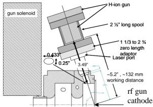
Figure 1: Layout of the ion gun and rf gun. The gun is installed on a laser port with a direct line of site to the cathode.
