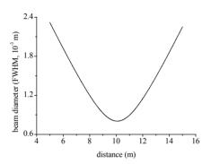
Figure 3: Seed laser beam diameter as a function of the distance to the focusing telescope showing a focus of 0.8 mm diameter (FWHM) inside the modulator.
