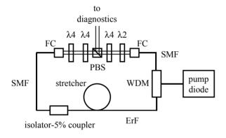
Figure 2: Schematic view of the Erbium fiber oscillator. FC: fiber coupler; SMF: single mode fiber; ErF: Erbium doped fiber, PBS: polarising beam splitter, WDM: wavelength division multiplexer,  $\lambda 4$ : quarter lambda plate,  $\lambda 2$ : half lambda plate.
