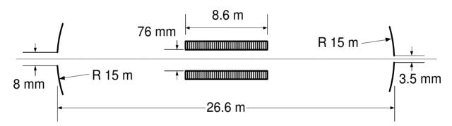
Figure 3: Scheme of the optical resonator.
