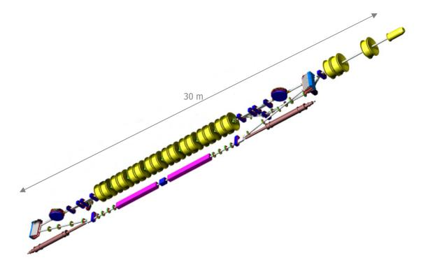
Figure 2: Scheme of the first stage of the Novosibirsk terahertz FEL. The loop lies in the vertical.
