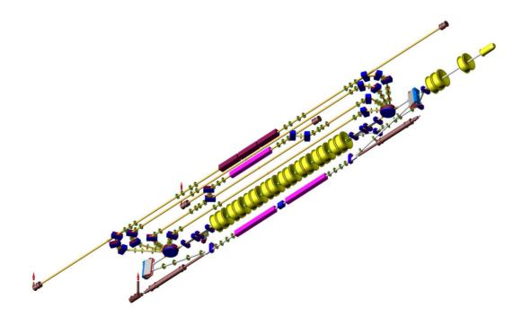
Figure 6: Scheme of the second stage of the Novosibirsk terahertz FEL. The terahertz FEL orbit lies in the vertical plain. Other four orbits lie in the horizontal one.
