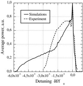
Figure 4: Dependence of the average power on the RF frequency detuning.
