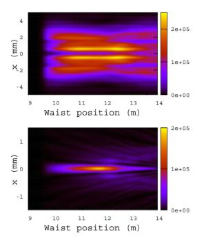
Figure 7: Intensity (a. u.) cross sections in the far field (top) and at the undulator entrance (bottom) as a function of the waist position of the cold-cavity fundamental mode of the resonator. The hole radius is 2mm.
