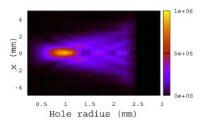
Figure 8: Intensity (a. u.) cross section in the far field as a function of hole radius, for waist position 12.19m.
