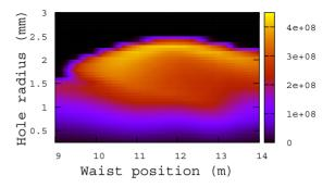
Figure 5: Output power (W) as a function of hole radius and waist position.
