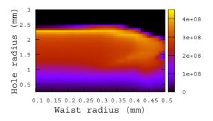
Figure 6: Output power (W) as a function of hole radius and waist size, for waist position 12.19m.
