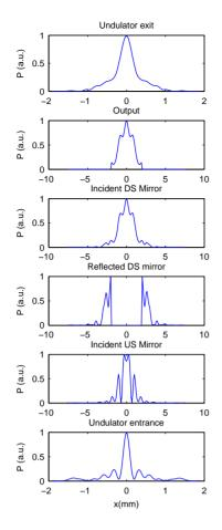
Figure 3: The normalised intensity cross sections at saturation, for different points within the optical cavity. The parameters are the CDR values (waist position 12 m, waist radius 0.34mm).
