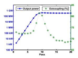
Figure 2: The growth of output power and the measured outcoupling fraction, both as a function of pass number, for the CDR parameters.
