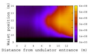
Figure 9: Power (W) growth along undulator as a function of waist position. The vertical bands are due to the gaps between the undulator sections.
