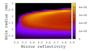
Figure 4: Output power (W) as a function of hole radius and mirror reflectivity. The CDR hole radius is 2mm and mirror reflectivity is 60%.
