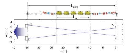
Figure 1: A schematic of the 4GLS VUV-FEL with the baseline CDR parameters. The fundamental cavity mode is shown on the same longitudinal scale as the engineering representation. The electron beam direction is right to left.
