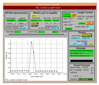
Figure 6. Detuning curve taken through a spectrometer set to 935 nm. The lasing occurs over about 0.5 microns in cavity length. The fundamental is not lasing over this range.
