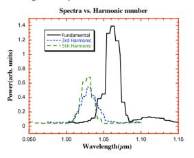
Figure 2. Spectra while lasing with 1.06 micron mirrors with the resonant wavelength equal to 1.02, 3.06, and 5.1 microns. The resonator losses were 3.5%/pass. Note the movement towards 1.02 microns as the harmonic number is increased.
