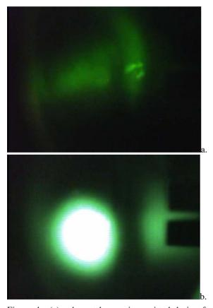
Figure 4. (a) coherent harmonics emitted during fundamental lasing on the output coupler of the laser. (b) Harmonic lasing at 0.53 microns obtained by lengthening the optical cavity by a fraction of a micron.
