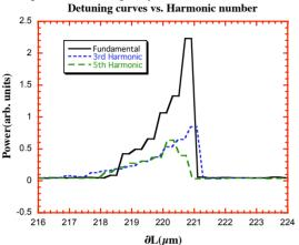
Figure 1. Power vs. cavity length for lasing at the fundamental, third, and fifth harmonic, with fundamental wavelength  $\sim 1.04 \ \mu$ m.
