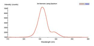
Figure 5. Lasing spectrum using an Ocean Optics visible spectrometer array. This is a single macropulse shot.
