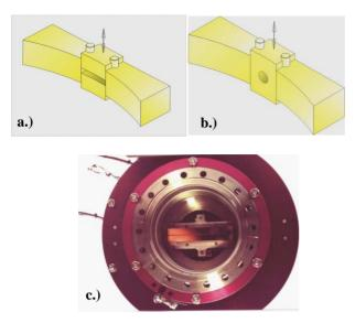
Figure 2 a-c: The lateral dimension of the outcoupler mirrors shown in a.) , b.) amounts to ~14 cm. The radius of curvature is ~3.5 m. The outcoupler mirror shown in c.) is constructed for an FIR FEL operating at ~230-650  $\mu$ m.
