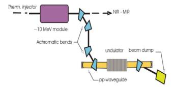
Figure 1: Layout of the FIR-FEL beamline option.
