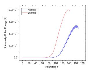
Figure 4: FEL operation at 13 MHz and 26 MHz pulse rep. rates with ~5.8 m cavity length ,  $\lambda$  ~ 155  $\mu$ m.
