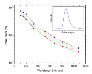
Figure 3: The upper peak power values (blue dots) are obtained at the peak of the detuning curve whereas the lower data points at cav. Detuning  $\sim -0.4 \cdot \lambda$ .
