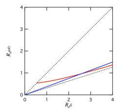
Figure 2: Dispersion relations of the evanescent wave for  $TM_{01}$  mode. The relative dielectric constant of the medium is 10.(red) Both axes are multiplied by the channel radius ( $R_d$ =25  $\mu$ m) for the normalization. The blue solid line shows the dispersion of 40 keV beam mode. Upper and lower dashed lines denote the dispersion of the light in vacuum and the light in the dielectric medium, respectively.
