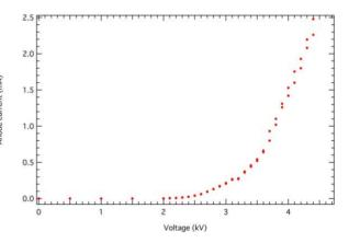
Figure 8: V-I curve for carbon nanotube cathode. D.C. voltage up to 4.4 kV was applied to the collector electrode.
