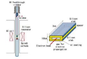
Figure 4: Schematic view of the CFEL test bench and the resonator. The left and right figures show the schematic view of the whole system and the detailed view of the resonator, respectively.
