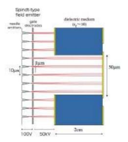
Figure 1: Schematic view of compact CFEL.
