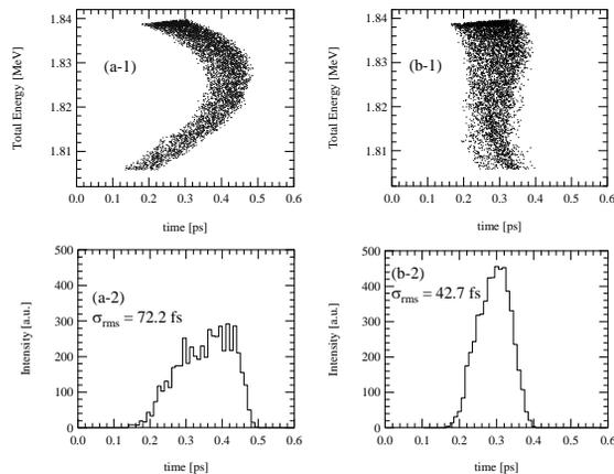
Figure 5. longitudinal phase space distributions and time distributions after bunch compression. (a-1), (a-2)  $\alpha$ -magnet case, (b-1), (b-2) TBA lattice case.
