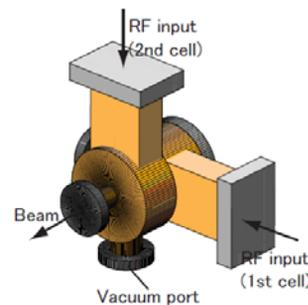
Figure 1. The prototype of ITC-RF gun. The RF input port is separated each other. This is now under manufacturing.
