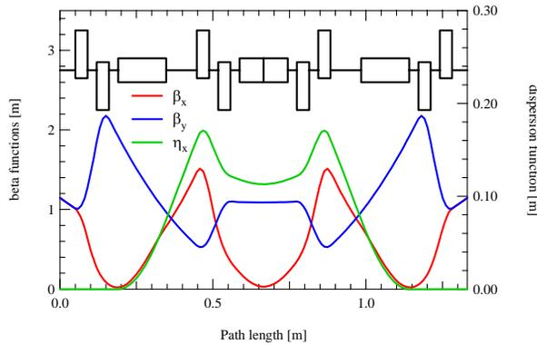
Figure 4. TBA optics. Left axis is for beta functions. Right axis is for dispersion function.
