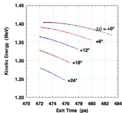
Figure 2. longitudinal phase space.  $\Delta\theta$  is a variable in this simulation.  $(E_1, E_2) = (25, 50)$  MV/m.
