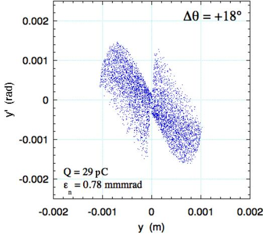
Figure 3. transverse phase space.  $(E_1, E_2) = (25, 50)$  MV/m,  $\Delta\theta = +18$  degree.
