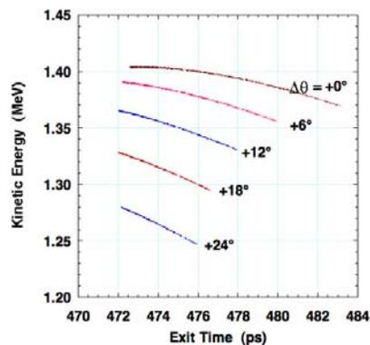
Figure 2. longitudinal phase space.  $\Delta\theta$  is a variable in this simulation.  $(E_1, E_2) = (25, 50)\ \text{MV}/\text{m}$ .
