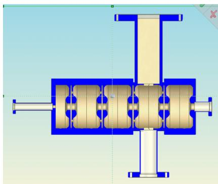
Fig.5: the schematic of the photo-cathode injector.
