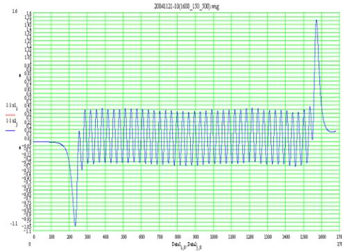
Fig.10: simulation trajectory of the electron in the wiggler.
