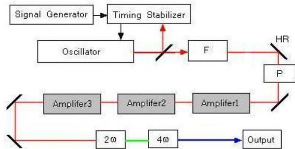
Fig.8: Optical Schematic of the cathode-driving laser system F, the Flady isolator.P, pockel .HR, high reflector.
