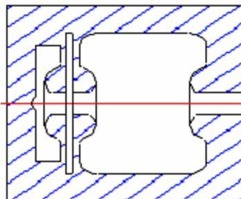
Fig.2: the schematic of the thermionic cathode injector.
