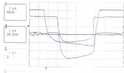
Fig.12: the beam current at the different position on the beam line, measured with BCT.
