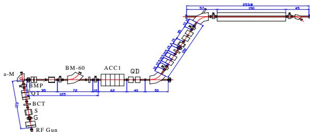
Fig.1: the schematic of the FIR-FEL facility.
