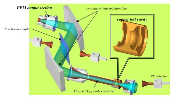
Figure 4: Schematic diagram of the test facility for studying surface heating effects based on JINR-IAP FEM.
