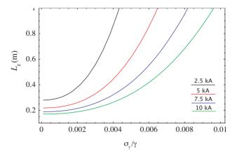
Figure 1: Exponential gain length as a function of incoherent energy spread for various electron beam currents as determined from the Xie [12] empirical fitting function.
