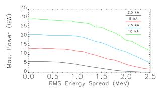
Figure 2: Predicted (GINGER calculations) maximum power in amplifier mode (with 15 MW initial HHG seed) over the THUNDER undulator (5 m) as a function of initial incoherent energy spread for various beam currents.
