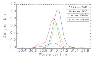
Figure 5: Predicted (GINGER calculations) output spectra at the 31-nm wavelength fundamental for the various SASE and seeded cases. Each bin is  $64.6\,\mathrm{meV}$  wide while 1 GW is equivalent to  $1.0\times10^{13}\,\mathrm{photons}.$
