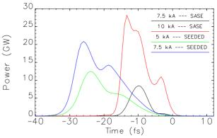
Figure 4: Predicted (GINGER calculations) output power temporal profiles for the cases associated with Fig. 3. The electron beam center is at t=0.
