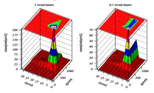
Figure 5: Radiation doses inside the magnets induced by a 1nC electron bunch hitting the vacuum chamber. The data are averaged over the  $0^{\circ}$ ,  $45^{\circ}$  and  $90^{\circ}$  scenarios.
