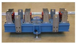
Figure 2: Electromagnetic Chicane.
