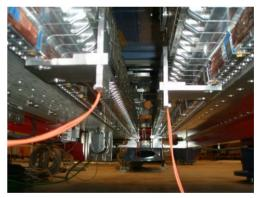
Figure 1: Radiator of the APPLE II type in operating position without vacuum chamber. Four power meter sensors (see below) at each undulator end (orange cable) are installed.
