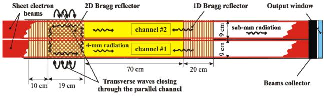
Fig. 5 Scheme of two-stage generation for the band of 0.1–0.3 mm
