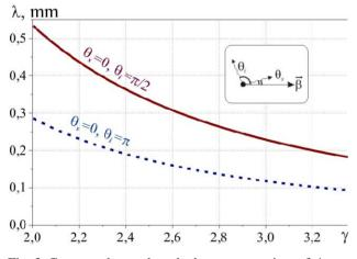
Fig. 2 Conversed wavelength due to scattering of 4-mm radiation on beam electrons as the function of the beam  $\gamma$ -factor
