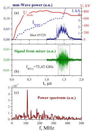
Fig. 1 Single frequency operation of 4-mm FEM: a) diode voltage ( $U_{diode}$ ), beam current ( $I_{beam}$ ) and mm-wave power; b) intercarrier frequency signal from heterodyne mixer (heterodyne frequency f<sub>drive</sub>=75.43 GHz); c) mm-wave power spectrum.
