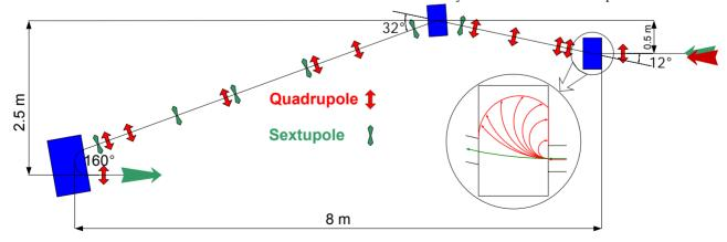
Figure 2. The layout of the first bent.
