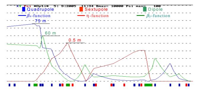
Figure 3. The lattice functions in the first bent.
