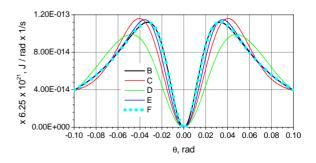
Fig. 1. Angular distribution of the backward TR for different wavelengths and 15 MeV electrons. C-  $\lambda$ =1 mm, far-field zone; D-  $\lambda$ =1 mm, R=250 mm; E-  $\lambda$ =0.3 mm,
