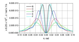
Fig. 2. Angular distribution of the backward TR for different wavelengths and 40 MeV electrons. C-  $\lambda$ =1 mm, far-field zone; D-  $\lambda$ =1 mm, R=250 mm; E-  $\lambda$ =0.3 mm, R=250 mm; F-  $\lambda$ =0.1 mm, R=250 mm. Curve B was computed using Ginzburg-Frank formula.
