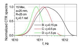
Fig. 3. Calculated normalized CTR spectra for 15 MeV for different  $\sigma_t$  at a=25 mm,  $\theta_0=0.1$  rad.
