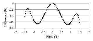
Figure 3. A polynomial fit is made for each Hall probe calibration. The polynomial coefficients are applied to measured data to calculate the corrected field. The difference between two Hall probe calibrations is shown.
