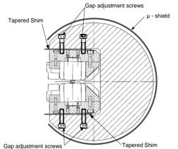
Figure 2. Each undulator is wrapped in a mu-shield, which reduces the ambient magnetic field effect by a factor of 6.
