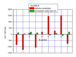
Figure 3: Distribution of the first field integral in the regular undulator periods (Io=200 A) before and after correction
