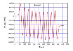
Figure 8: Magnetic field second integral for Io=435 A
