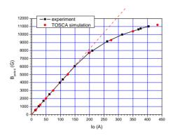
Figure 2: Undulator magnetization curve
