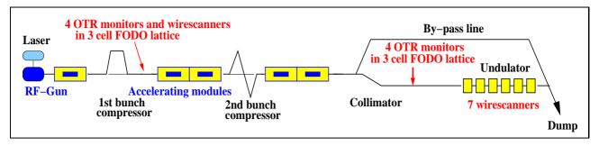
Figure 1: Layout of the FLASH linac (not to scale). Beam direction is from left to right, and the total length is about 250 m. Locations of OTR monitors and wire scanners, used for the emittance measurements, are indicated.
