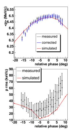
Figure 2: Mean momentum (top) and momentum spread (bottom) as a function of the gun phase.
