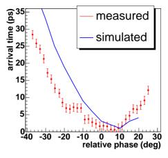
Figure 6: Relative arrival time of the bunch at the streak camera.
