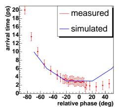
Figure 8: Relative arrival time of the photon pulse produce by the electron bunch at the streak camera as a function of the booster phase. This is assumed to be equal with arrival time of the electron bunch at the screen station
