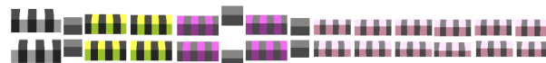
Figure 4: Layout of FERMI FEL-2 in superradiant cascade mode. Similarly to the case of FEL-1, the first modulator and two radiators of the first stage are used to prepare a modulated beam with the features shown in Fig. 2 at harmonic 5. The last radiator of the first stage and the modulator of the second stage are tuned to harmonic 10 while the entire final radiator is tuned to harmonic 30 to reach the final wavelength of \lambda = 7.7 nm.
