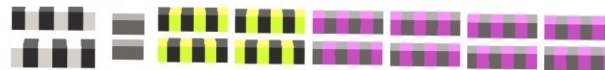
Figure 1: Layout of FERMI FEL-1. The modulator (period length of \lambda_m = 10 cm) is tuned to the seed wavelength ( \lambda_s = 232 nm). The amplifier is composed of two parts. Two undulators are resonant with the 5th harmonic of the seed ( \lambda_1 = 46 nm) and the last four undulators are tuned to the 10th ( \lambda_f = 23.2 nm) or 15th ( \lambda_f = 15.6 nm) harmonics of the seed.
