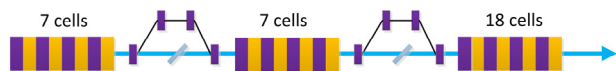
Figure 1: Design of LCLS-II hard X-ray baseline undulator system including two ‘miss undulators’ which are reserved for self-seeding operation.
