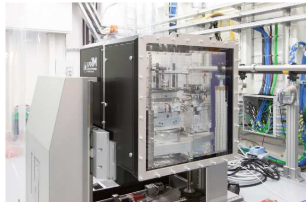
Figure 9: Large Pixel Array detector in the FXE experimental hutch.
