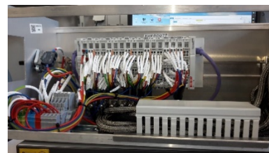
Figure 6: Assembly of a PLC module at NCBJ.
