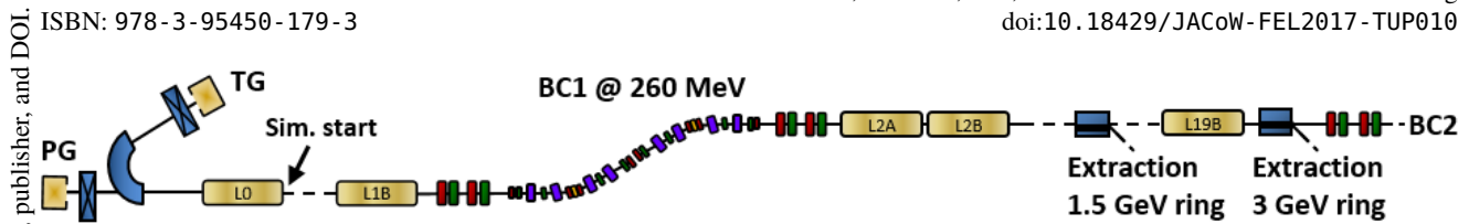
Figure 1: Compact layout of the MAX IV Linac. Yellow denotes radiofrequency (RF) structures, red/green are focusing/defocusing quadrupole magnets, purple are dipole magnets, orange are sextupole magnets and blue are special magnets. PG and TG are photo-cathode and thermionic RF guns, respectively, L are the linac sections and BC1 is the first bunch compressor. This view is cut right before BC2, which is shown in Fig. 2.
