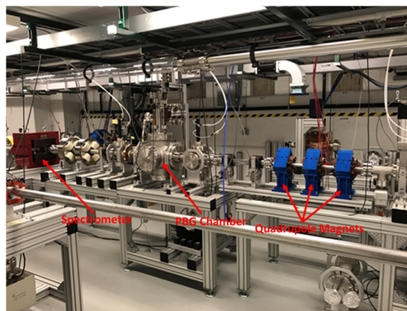
Figure 1: The experimental setup on the beam line at Argonne Wakefield Accelerator (AWA).
