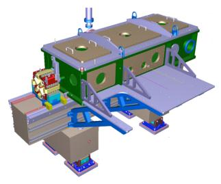
Figure 2: 3D model of the ACHIP chamber in the SwissFEL switchyard.
