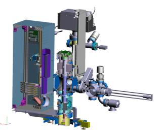
Figure 1: 3D breakout model of the ACHIP injector chamber.
