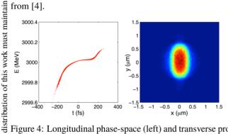
Figure 4: Longitudinal phase-space (left) and transverse pro-N file (right) of the simulated electron beam at the experiment location. The rms pulse duration is 92 fs, the rms energy 8 spread is 42 keV, and the rms beam sizes are 0.26 µm (hori-201 zontal) and 0.36 µm (vertical) Image reproduced from [4]. O
