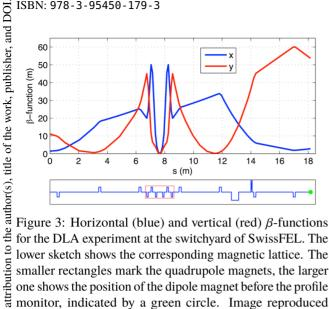
Figure 3: Horizontal (blue) and vertical (red)  $\beta$ -functions for the DLA experiment at the switchyard of SwissFEL. The lower sketch shows the corresponding magnetic lattice. The smaller rectangles mark the quadrupole magnets, the larger one shows the position of the dipole magnet before the profile monitor, indicated by a green circle. Image reproduced from [4].
