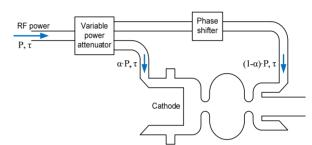
Figure 1: A schematic of the proposed two-cell photoinjector.
