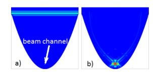
Figure 4: Field distributions at the parabolic mirror while focusing the short THz pulse, for the time correspondent to beginning of focusing at t=5 ps (a) and for time when focusing is close to maximum at t=33 ps (b).
