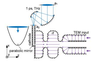
Figure 3: RF gun wherein electron emission is controlled by a picosecond THz pulse irradiating a metallic cathode.
