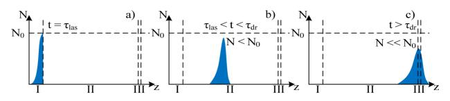
Figure 9: Free carrier packet dynamics in the layered diamond. Three snapshots are illustrated: (a) just-formed electron pulse upon the absorption of the laser pulse (b) electron pulse drift in the external electric field toward the NEA surface. and (c) onset of emission into vacuum.
