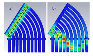
Figure 7: Concept for particle acceleration by a single picosecond THz pulse propagating in periodic accelerating gaps.
