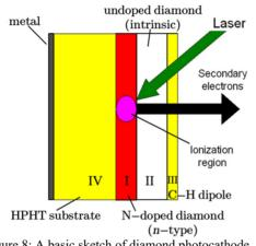
Figure 8: A basic sketch of diamond photocathode.
