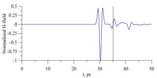
Figure 6: Magnetic field components at the focus of the parabolic mirror.
