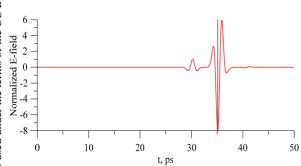
Figure 5: Electric field components at the focus of the parabolic mirror.
