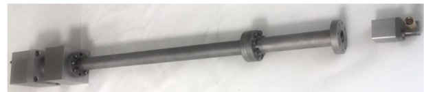
Figure 8: A 34-GHz TE_{11} - TE_{21} - TM_{11} RF undulator and a low-power experimental setup.
