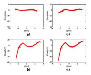
Figure 2: High order energy spread along the injector, (a) at the middle of the buncher;
