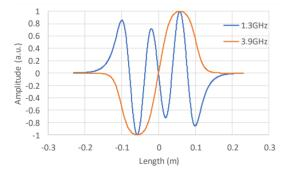
Figure 3: Fundamental and Harmonic electric field along the axis of the buncher.
