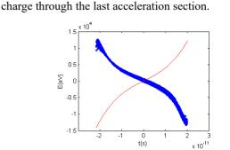
Figure 4: Correction of the high order energy modulation by harmonic cavity. Blue dots represent the longitudinal distribution at the entrance of the buncher. Red line is the combined electric field of two modes.
