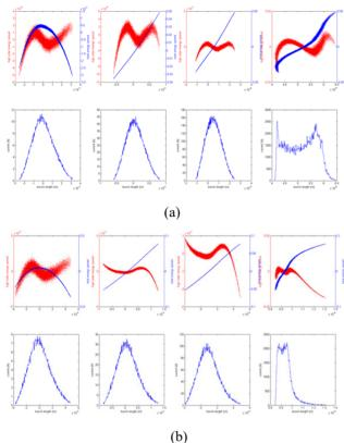
3.0 licence (@ 2019). Any distribution of this work must maintain attribution to the author(s), title Figure 6: Longitudinal phase space along the linac (method 2). (a) bunch length is 1.1 mm (original design) at the ВΥ injector exit; (b) bunch length is 1.6 mm at the injector Content from this work may be used under the terms of the CC exit.
