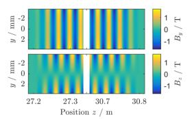
Figure 1: Magnetic field map used in the simulations. Only a small section including the entrance and exit of the 3.6 m long undulator model is shown.
