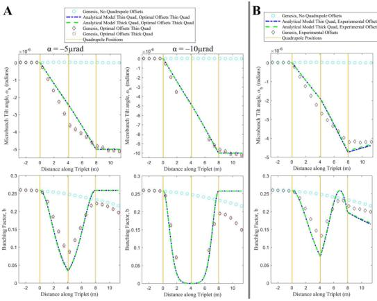
Figure 2: Microbunch tilt angle in nonrotated frame,  $\alpha_b$  and bunching factor, b, through an quadrupole triplet. are A) analytical model optimal using thin or thick quadrupoles, or B) replicating a 2018 experiment.
